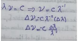
B- For a Nd:YAG laser with a central frequency 1.06  $\mu$ m and frequency linewidth  $\Delta v = 1.2 \times 10^{11}$  Hz, calculate the spectral linewidth of such a laser.
